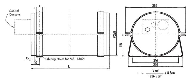
The connection fittings and the control unit can only be assembled on the face of the end cap. For each 5 litres of gas volume one 1/2" - 20 BS 150 safety plug must be used. If the control console is mounted to the tank, its internal safety plug can be counted as one plug.
