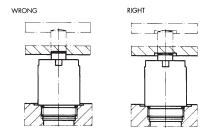
Any lateral clamping of the piston rod dramatically reduces the cylinder lifetime. The position rod must remain laterally free.
