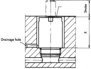
When cylinders are embedded in the manifold plate, a drainage hole must be drilled in the bottom of the pocket to prevent the accumulation of oil and other debris.
