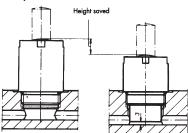
If space permits, the tool height can be reduced by using low profile or pancake cylinders (CDSN or CDSK).
